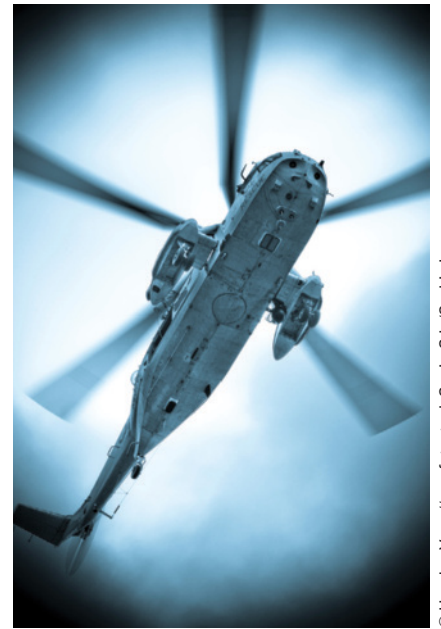
The blades of a helicopter impart downward momentum to a column of air, thereby creating the forces necessary for hovering and maneuvering.
