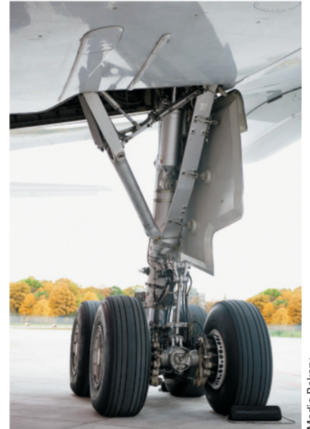
Portions of the landing gear for a large aircraft undergo three-dimensional motion during retraction and deployment.
