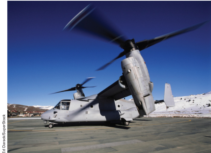
The engine/propeller units at the wingtips of this V-22 Osprey can tilt from a vertical takeoff position to a horizontal position for forward flight.
